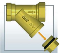
Unscrew the terminal plug with a 19 mm key for a 1/2" strainer or with a 21 mm key for 3/4" and 1" strainers.
